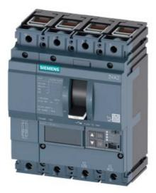
CIRCUIT BREAKER 3VA2 IEC FRAME 160 BREAKING CAPACITY CLASS M ICU=55KA @ 415 V 4POLE, LINE PROTECTION ETU850, LSI, IN=40A OVERLOAD PROTECTION IR=16A ...40A SHORT CIRCUIT PROTECTION ISD=0,6..10X IN, II=1,5..12X IN NEUTRAL PROTECTION ADJUSTABLE (OFF, UPTO 160%) CABLE CONNECTION
