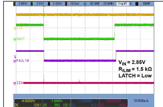
FIGURE 2-16: Output Recovery from Short Circuit.
