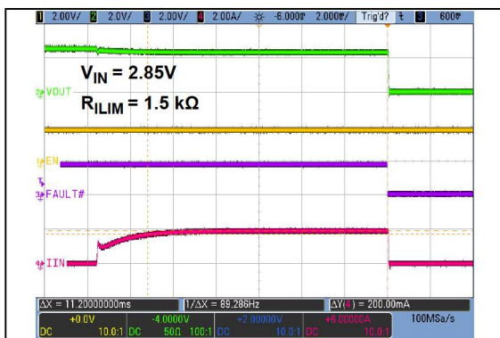
FIGURE 2-3: Overcurrent Fault Response Delay Time.
