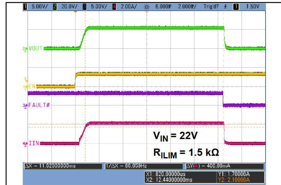
FIGURE 2-4: Overcurrent Fault Response Delay Time.
