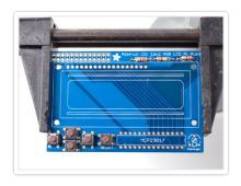
Next up we will place the buttons. These buttons are useful to send a signal to the Pi (say if you have a basic menu system). We have a 4-way 'direction pad' for up/down/left/right input and a button to the right called SELECT. These 5 buttons should be able to make 'talking' back to your project easy. These are connected to the I2C port expander chip so they require no extra pins on the Pi, our library does the work of reading whether they are pressed.
