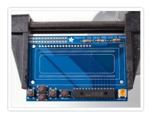
We're nearly done! Now we will place the I2C port expander chip. Double check that it has the MCP23017-E/SP marking on it. This is a 16-pin expander chip, that uses the i2c bus. That means you can send it commands using the i2c pins on an Pi and control 16 more digital pins! 5 of those pins go to the buttons, 6 go to the LCD control and 3 are used for the backlight (the remaining 2 are unused).
