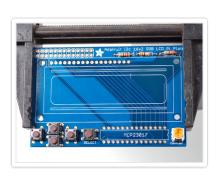
Next, place the 10K potentiometer (the orange-faced thing with three legs) into the spot above the RESET button. It will only fit one way. This is the contrast potentiometer which will adjust how dark the characters appear. All displays are slightly different so you'll adjust this once the display is soldered in.
