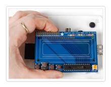
Place the 2x13 header onto your Pi, and slide the plate on top, it should fit perfectly.
