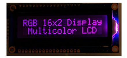
You can also use 16x2 LCDs or even OLEDs that are the same size that do not have an RGB backlight, or have no backlight at all.
