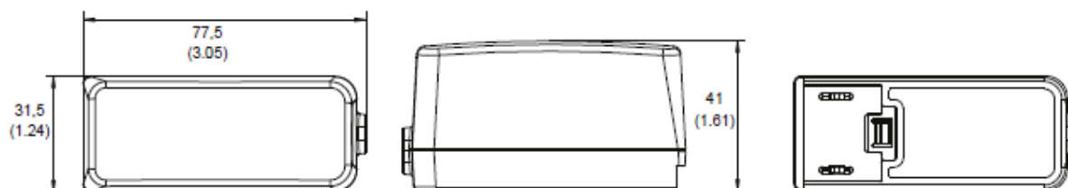
Alle Abmessungen in Millimeter (Inch), Abweichung ± 0,5 (0.02) All Dimensions in Millimeter (Inch), Deviation ± 0,5 (0.02)
