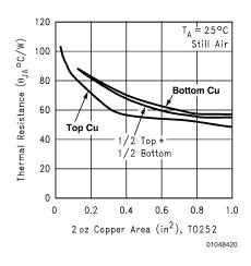
FIGURE 3.  $\theta_{\text{JA}}$  vs. 2oz Copper Area for TO-252
