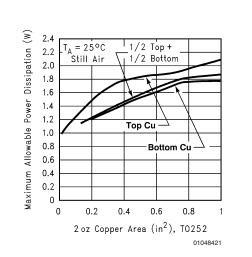
FIGURE 5. Maximum Allowable Power Dissipation vs. 20z. Copper Area for TO-252
