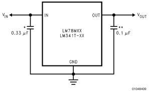
\*Required if regulator input is more than 4 inches from input filter capacitor (or if no input filter capacitor is used).
