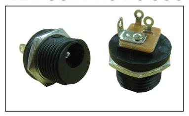
This round style DC socket has an M12.7 thread and is available with either Ø2.1mm or Ø2.5mm pin. Supplied with nut.
