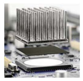
Low thermal contact resistances can be achieved with a very reliable adhesive strength on different surfaces.
