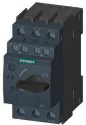
CIRCUIT-BREAKER SZ S0, FOR MOTOR PROTECTION, CLASS 10, A-RELEASE 13...20A, N-RELEASE 260A, SCREW CONNECTION, STANDARD SW. CAPACITY, W. TRANSVERSE AUX. SWITCH 1NO+1NC
