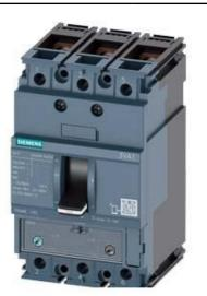
CIRCUIT BREAKER 3VA1 IEC FRAME 160 BREAKING CAPACITY CLASS H ICU=70KA @ 415 V 3-POLE, LINE PROTECTION TM240, ATAM, IN=20A OVERLOAD PROTECTION IR=14A ...20A SHORT CIRCUIT PROTECTION II=5...10 X IN BUSBAR CONNECTION
