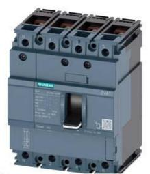
CIRCUIT BREAKER 3VA1 IEC FRAME 160 BREAKING CAPACITY CLASS S ICU=36KA @ 415 V 4-POLE, LINE PROTECTION TM210, FTFM, IN=80A OVERLOAD PROTECTION IR=80A FIXED SHORT CIRCUIT PROTECTION II=10 X IN NEUTRAL UNPROTECTED BUSBAR CONNECTION
