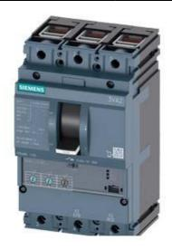
CIRCUIT BREAKER 3VA2 IEC FRAME 100 BREAKING CAPACITY CLASS L ICU=150KA @ 415 V 3POLE, LINE PROTECTION ETU320, LI, IN=25A OVERLOAD PROTECTION IR=10A ...25A SHORT CIRCUIT PROTECTION II=12 X IN CABLE CONNECTION
