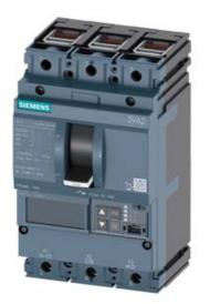
CIRCUIT BREAKER 3VA2 IEC FRAME 160 BREAKING CAPACITY CLASS C ICU=110KA @ 415 V 3POLE, LINE PROTECTION ETU860, LSIG, IN=160A OVERLOAD PROTECTION IR=64A ...160A SHORT CIRCUIT PROTECTION ISD=0,6..10X IN, II=1,5..10X IN NEUTRAL PROTECTION OPTIONAL WITH EXT. CT,UPTO 160% GROUNDFAULT, SWITCHABLE IG=0,2... 1 X IN, TG=0,050,8MS CABLE CONNECTION
