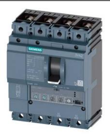
CIRCUIT BREAKER 3VA2 IEC FRAME 250 BREAKING CAPACITY CLASS L ICU=150KA @ 415 V 4POLE, LINE PROTECTION ETU330, LIG, IN=160A OVERLOAD PROTECTION IR=64A ...160A SHORT CIRCUIT PROTECTION II=1,5...12 X IN NEUTRAL PROTECTION ADJUSTABLE(OFF,50%,100%) GROUNDFAULTPROTECTION IG=0,2... 1 X IN, TG=0,1/0,3MS BUSBAR CONNECTION
