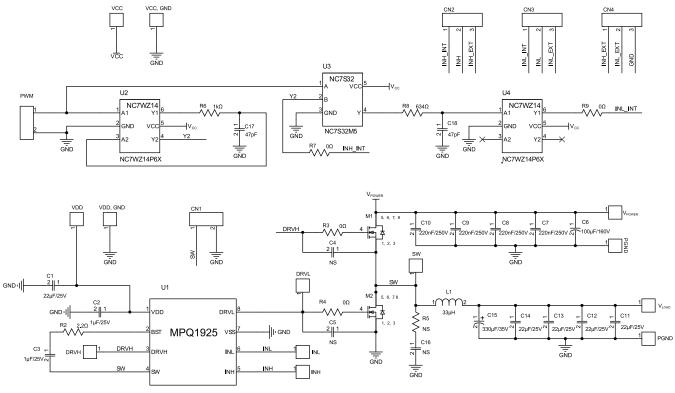
Figure 2: Evaluation Board Schematic
