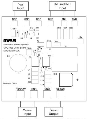
Figure 1: Test Set-Up for the EVQ1925-R-00A
