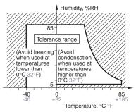
\* -40 to  $+85^{\circ}$ C -40 to  $+185^{\circ}$ F (When 45% to 80%V of coil holding voltage)
