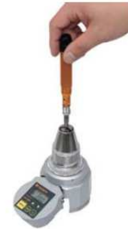
Torque checking figure for BMRD torque screwdriver for small screws with BTGE-G
