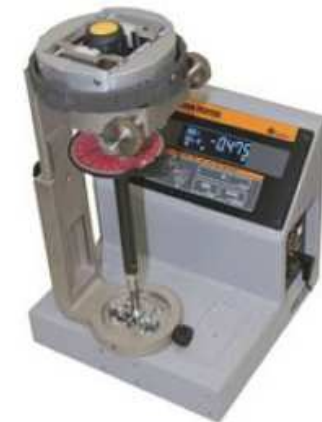
Calibration figure for torque screwdriver RTD left and FTD right with TDT3-G
