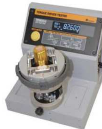
Calibration figure for torque screwdriver RTD left and FTD right with TDT3-G
