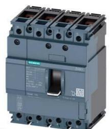
CIRCUIT BREAKER 3VA1 IEC FRAME 100 BREAKING CAPACITY CLASS N ICU=25KA @ 415 V 4-POLE, LINE PROTECTION TM210, FTFM, IN=80A OVERLOAD PROTECTION IR=80A FIXED SHORT CIRCUIT PROTECTION II=10 X IN NEUTRAL UNPROTECTED BUSBAR CONNECTION
