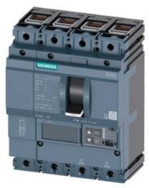
CIRCUIT BREAKER 3VA2 IEC FRAME 160 BREAKING CAPACITY CLASS C ICU=110KA @ 415 V 4POLE, LINE PROTECTION ETU550, LSI, IN=100A OVERLOAD PROTECTION IR=40A ...100A SHORT CIRCUIT PROTECTION ISD=0,6..10X IN, II=1,5..12X IN NEUTRAL PROTECTION ADJUSTABLE (OFF, UPTO 160%) CABLE CONNECTION
