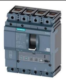
CIRCUIT BREAKER 3VA2 IEC FRAME 160 BREAKING CAPACITY CLASS C ICU=110KA @ 415 V 4POLE, LINE PROTECTION ETU330, LIG, IN=63A OVERLOAD PROTECTION IR=25A ...63A SHORT CIRCUIT PROTECTION II=1,5...12 X IN NEUTRAL PROTECTION ADJUSTABLE(OFF,100%) GROUNDFAULTPROTECTION IG=0,2... 1 X IN, TG=0,1/0,3MS CABLE CONNECTION
