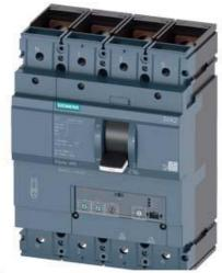
CIRCUIT BREAKER 3VA2 IEC FRAME 400 BREAKING CAPACITY CLASS H ICU=85KA @ 415 V 4-POLE, LINE PROTECTION ETU320, LI, IN=400A OVERLOAD PROTECTION IR=160A ...400A SHORT CIRCUIT PROTECTION II=10 X IN NEUTRAL PROTECTION ADJUSTABLE(OFF,50%,100%) BUSBAR CONNECTION
