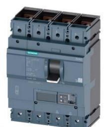
CIRCUIT BREAKER 3VA2 IEC FRAME 630 BREAKING CAPACITY CLASS H ICU=85KA @ 415 V 4-POLE, LINE PROTECTION ETU860, LSIG, IN=500A OVERLOAD PROTECTION IR=200A ...500A SHORT CIRCUIT PROTECTION ISD=0,6..10X IN, II=1,5..14X IN NEUTRAL PROTECTION ADJUSTABLE (OFF, UPTO 100%) GROUND-FAULT, SWITCHABLE IG=0,2... 1 X IN, TG=0,05-0,8MS BUSBAR CONNECTION
