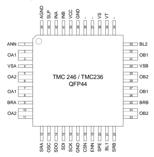
Figure 2.1 TMC246 pin assignments
