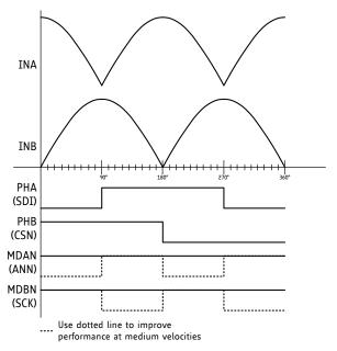
Figure 5.1 Analog control for standalone mode
