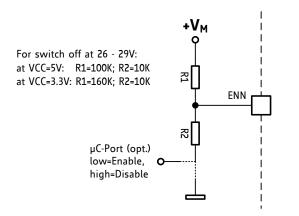
Figure 9.1 Overvoltage protection example for limiting to 30V
