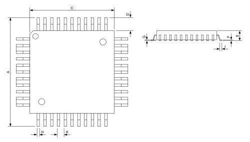
Figure 15.1 Dimensional drawings (PQFP44)
