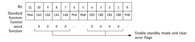
Programming current value 0000 for both coils at a time clears the overcurrent flags and switches the TMC246 into a low current standby mode with coils switched off.
