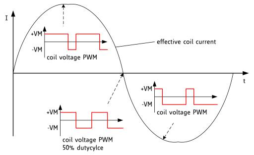
Figure 7.3 Voltage PWM generates motor current
