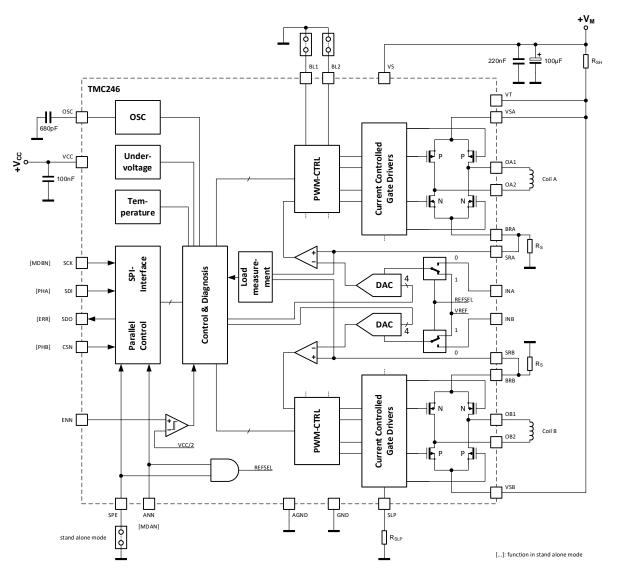
Figure 1.1 TMC246 block diagram
