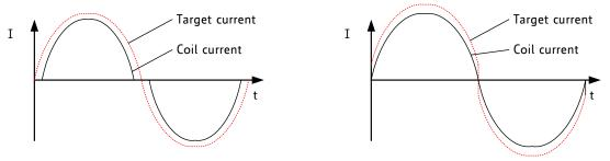
Coil current does not have optimum shape
