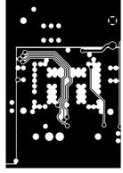
The layout example is shown to demonstrate the principle of a compact layout with large heat spreading areas for all motor outputs. The short to GND detection uses a voltage divider to allow simple adaptation of the triggering current. RC filtering is included for SRA and SRB for best performance.
