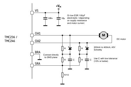
Figure 12.2 Driving a DC motor
