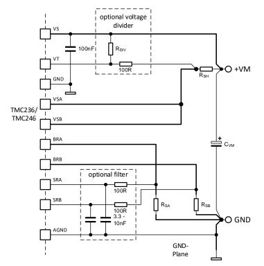
Figure 11.2 Grounding and power routing
