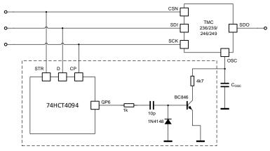
Figure 12.1 Synchronizing the chopper clock
