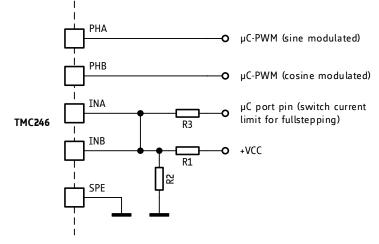
Figure 7.4 Controlling the driver with two PWMs in standalone mode
