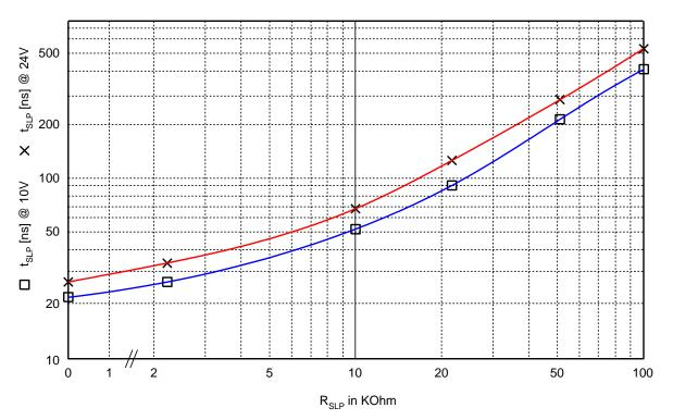
Figure 8.1 External R<sub>SLP</sub> controls switching slopes
