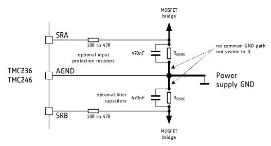
Figure 11.1 Sense resistor grounding and protection components
