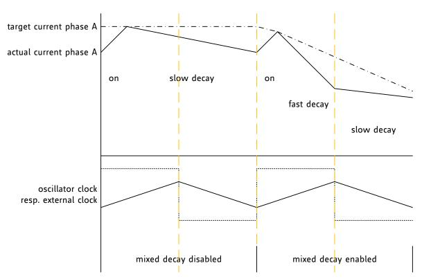
Figure 7.2 Chopper cycle showing use of mixed decay with falling current
