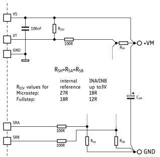
Figure 6.1 Schematic with R<sub>SH</sub>=R<sub>SA</sub>=R<sub>SB</sub>
