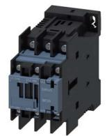
traction contactor, AC-3e/AC-3, 9 A, 4 kW / 400 V, 3-pole, 72 V DC, 0.7-1.25\* Us, electronic drive, with integrated varistor, auxiliary contacts: 1 NO + 1 NC, ring cable lug connection, size: S0
