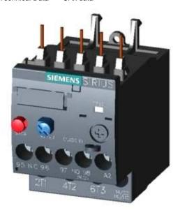
OVERLOAD RELAY 7.0...10 A FOR MOTOR PROTECTION SZ S00, CLASS 10, F. MOUNTING ONTO CONTACTOR MAIN CIRCUIT: SCREW TERMINAL AUX. CIRCUIT: SCREW TERMINAL MANUAL-AUTOMATIC-RESET
