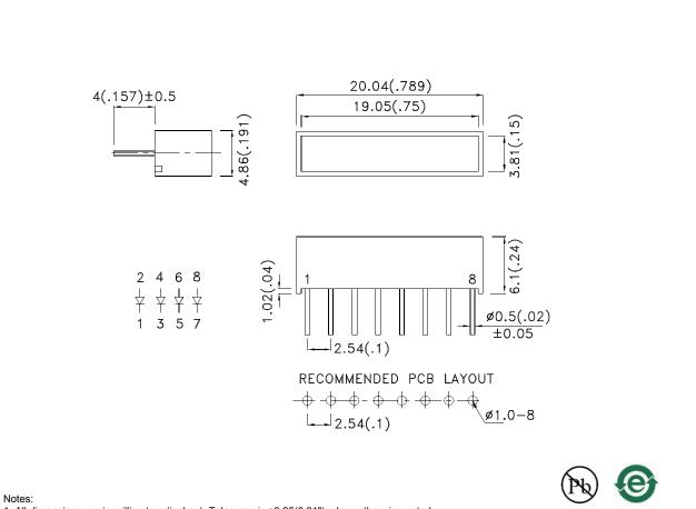
1. All dimensions are in millimeters (inches), Tolerance is ±0.25(0.01")unless otherwise noted.
