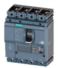
CIRCUIT BREAKER 3VA2 IEC FRAME 160 BREAKING CAPACITY CLASS C ICU=110KA @ 415 V 4POLE, LINE PROTECTION ETU850, LSI, IN=25A OVERLOAD PROTECTION IR=10A ...25A SHORT CIRCUIT PROTECTION ISD=0,6..10X IN, II=1,5..12X IN NEUTRAL PROTECTION ADJUSTABLE (OFF, UPTO 160%) BUSBAR CONNECTION
