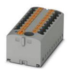
Distribution block, Basic terminal block with supply, nom. voltage: 500 V, nominal current: 24 A, connection method: Push-in connection, Push-in connection, number of connections: 7, cross section:0.14 mm² - 4 mm², AWG: 26 - 12, width: 25.2 mm, height: 21.2 mm, color: red, mounting type: for snapping onto a DIN rail adapter, Adapter plate
