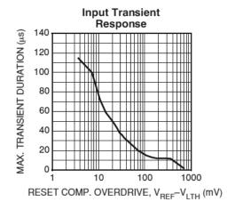
**Figure 4. Input Transient Response**
