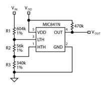
Figure 1. MIC841 Example Circuit
