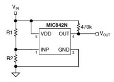
Figure 3. MIC842 Example Circuit
