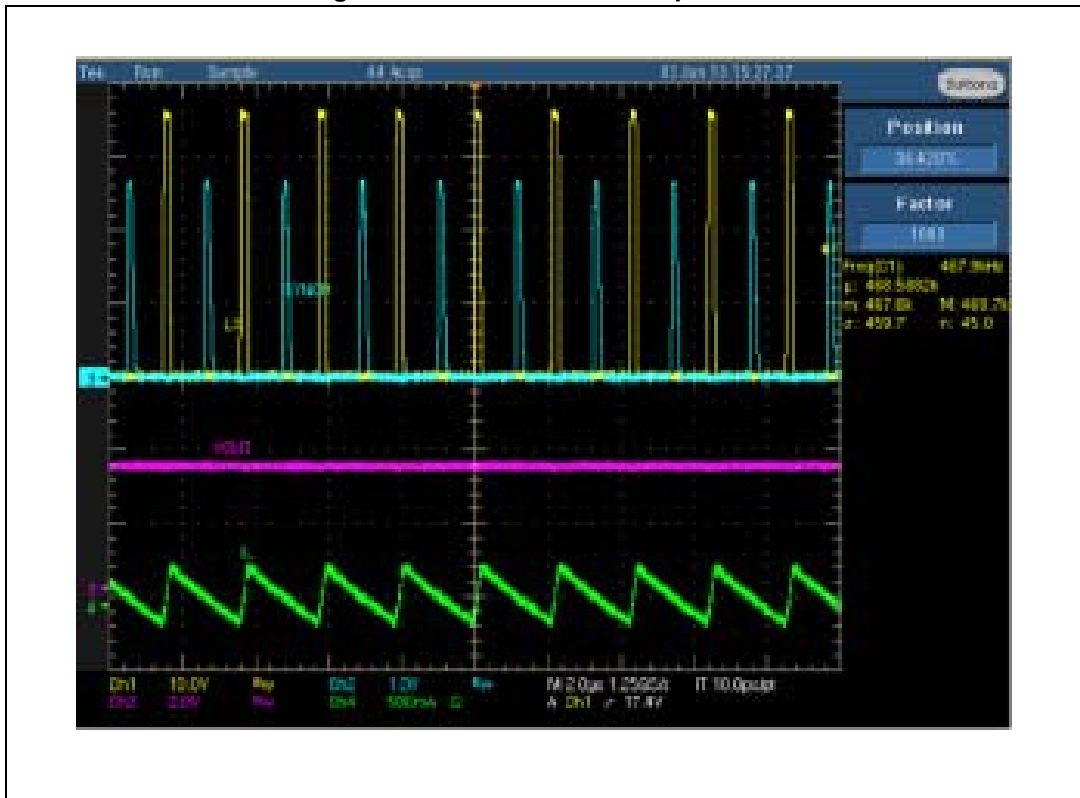
Figure 13. Low noise mode operation
