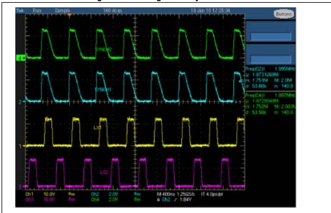
Figure 33. Two regulators synchronized
