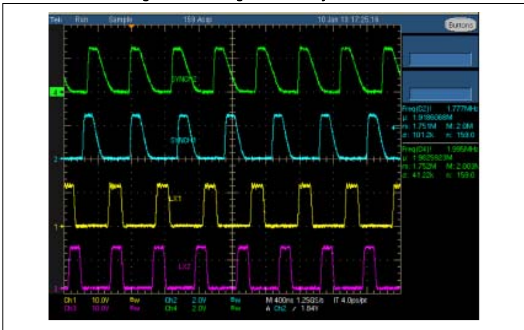
Figure 32. Two regulators not synchronized
