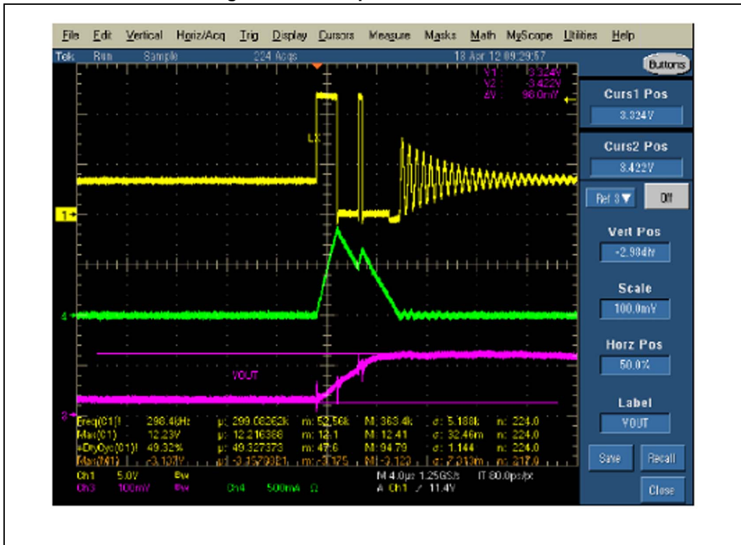
Figure 14. LCM operation at zero load
