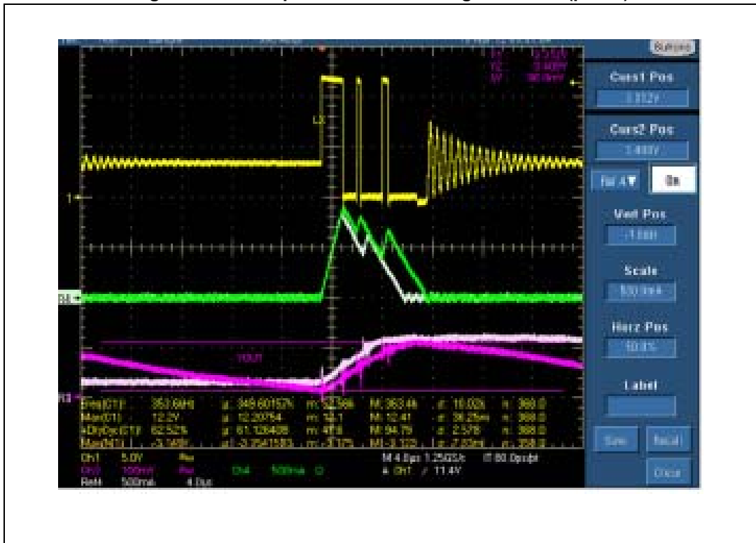
Figure 16. LCM operation over loading condition (part 2)
