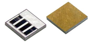
The high power back-contact resistor (IGBR) series thin film chip resistor utilizes the excellent thermal properties of silicon to allow ultra high power rating with miniature case size for hybrid (chip and wire) assemblies.
