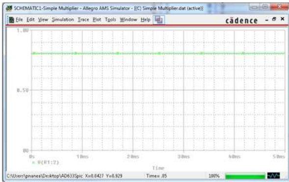
Figure 31. Simple Circuit Response Graph Displayed in PSPICE ( 2V \times 4V )/ 10V = 0.8V
