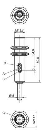
A Green LED B Yellow LED C Optical axis D Potentiometer
