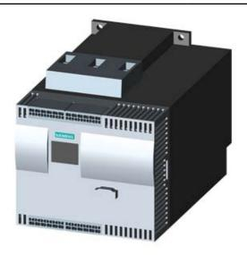
SIRIUS SOFT STARTER, VALUES WITH 460 V, 50 DEG., STANDARD: 32A, 20HP, INSIDE-DELTA CIRCUIT 3: 55A, 40HP, 200-460 V AC, 115 V AC, CAGE CLAMP TERMINALS
