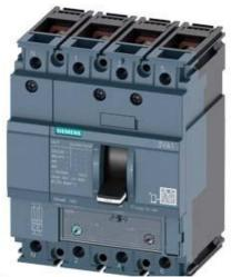
CIRCUIT BREAKER 3VA1 IEC FRAME 160 BREAKING CAPACITY CLASS N ICU=25KA @ 415 V 4-POLE, LINE PROTECTION TM240, ATAM, IN=100A OVERLOAD PROTECTION IR=70A ...100A SHORT CIRCUIT PROTECTION II=5...10 X IN NEUTRAL PROTECTION 100% BUSBAR CONNECTION
