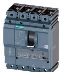
CIRCUIT BREAKER 3VA2 IEC FRAME 100 BREAKING CAPACITY CLASS L ICU=150KA @ 415 V 4POLE, LINE PROTECTION ETU350, LSI, IN=40A OVERLOAD PROTECTION IR=16A ...40A SHORT CIRCUIT PROTECTION ISD=1,5... 10 X IR, II=12 X IN NEUTRAL PROTECTION ADJUSTABLE(OFF,100%) BUSBAR CONNECTION
