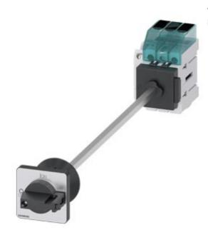
Switch disconnector 3LD3, main switch 3-polig, lu 25A operational switch at AC-23 A at 400 V 9,0 kW floor mounting Base mounting with door coupling center-hole 22,5 mm knob-operated mechanism black 48 x 48 mm with auxiliary 1NO+1NC
