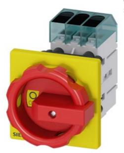
Switch disconnector 3LD3, main switch 3-polig, Iu 63A operational switch at AC-23 A at 400 V 22,0 kW front mounted Base mounting with center-hole 22,5 mm knob-operated mechanism red/yellow 66 x66 mm
