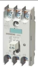
SOLID STATE RELAY 3-PHASE 3RF2 30 A 40 DEG. C  $48-600\ V\ /\ 4-30\ V\ DC\ 3PH.$ -CONTROLLED RING TERMINAL LUG BLOCKING VOLTAGE 1200 V
