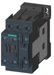
CONTACTOR, AC-3, 15KW/400V, 1NO+1NC, AC(50-60HZ)/DC ACTUAT. AC/DC 21...28V, 3-POLE, SZ S0 SCREW TERMINAL
