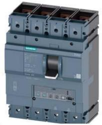
CIRCUIT BREAKER 3VA2 IEC FRAME 400 BREAKING CAPACITY CLASS M ICU=55KA @ 415 V 4-POLE, LINE PROTECTION ETU330, LIG, IN=250A OVERLOAD PROTECTION IR=100A ...250A SHORT CIRCUIT PROTECTION II=1,5...12 X IN NEUTRAL PROTECTION ADJUSTABLE(OFF,50%,100%) GROUND-FAULT-PROTECTION IG=0,2... 1 X IN, TG=0,1/0,3MS BUSBAR CONNECTION
