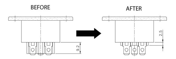
THIS MODIFICATION WILL NOT CHANGE THE FUNCTIONALITY, SAFETY, OR USE OF THIS PRODUCT IN ANYWAY. THE PRODUCT WILL FUNCTION 100% THE SAME, AND THE REDUCTION OF THE INSULATION WILL ALLOW FOR EASIER INSTALLATION.
