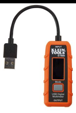
The Klein Tools ET900 is a USB digital meter for common standard USB-A (Type A) ports, including Qualcomm Quick Charge® ports. It accurately and reliably measures and displays the USB port voltage, current, capacity, energy and resistance simultaneously. It can function with any USB-A port that has the ability to deliver power. It requires NO batteries as it draws power from the power source to function.
