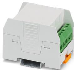
Empty enclosure for mounting on a DIN rail, light gray (7035), width: 45.1 mm, height: 77 mm, depth: 50.2 mm, incl. 2 PCB terminal blocks, 8-pos., screw connection, for 2.5 mm², nominal current: 24 A, 400 V, PCB surface: 2910 mm²
