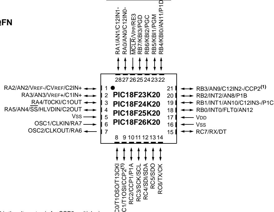
Note 1: RB3 is the alternate pin for CCP2 multiplexing.
