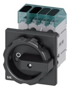
Switch disconnector 3LD3, main switch 3-polig + N, lu 63A operational switch at AC-23 A at 400 V 22,0 kW front mounted Base mounting with center-hole 22,5 mm knob-operated mechanism black  $66 \times 66$  mm
