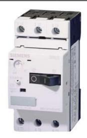
CIRCUIT-BREAKER SIZE S00, FOR MOTOR PROTECTION, CLASS 10, A-REL.2.2...3.2A, N-REL. 42A, SCREW TERMINAL, STANDARD SWITCHING CAPACITY
