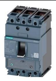
CIRCUIT BREAKER 3VA1 IEC FRAME 160 BREAKING CAPACITY CLASS N ICU=25KA @ 415 V 3-POLE, LINE PROTECTION TM240, ATAM, IN=125A OVERLOAD PROTECTION IR=87,5A ...125A SHORT CIRCUIT PROTECTION II=5...10 X IN BUSBAR CONNECTION
