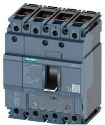
CIRCUIT BREAKER 3VA1 IEC FRAME 160 BREAKING CAPACITY CLASS S ICU=36KA @ 415 V 4-POLE, LINE PROTECTION TM240, ATAM, IN=125A OVERLOAD PROTECTION IR=87,5A ...125A SHORT CIRCUIT PROTECTION II=5...10 X IN NEUTRAL PROTECTION 100% BUSBAR CONNECTION
