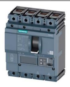
CIRCUIT BREAKER 3VA2 IEC FRAME 160 BREAKING CAPACITY CLASS L ICU=150KA @ 415 V 4POLE, LINE PROTECTION ETU860, LSIG, IN=100A OVERLOAD PROTECTION IR=40A ...100A SHORT CIRCUIT PROTECTION ISD=0,6..10X IN, II=1,5..12X IN NEUTRAL PROTECTION ADJUSTABLE (OFF, UPTO 160%) GROUNDFAULT, SWITCHABLE IG=0,2... 1 X IN, TG=0,050,8MS CABLE CONNECTION
