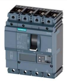
CIRCUIT BREAKER 3VA2 IEC FRAME 160 BREAKING CAPACITY CLASS C ICU=110KA @ 415 V 4POLE, LINE PROTECTION ETU560, LSIG, IN=40A OVERLOAD PROTECTION IR=16A ...40A SHORT CIRCUIT PROTECTION ISD=0,6..10X IN, II=1,5..12X IN NEUTRAL PROTECTION ADJUSTABLE (OFF, UPTO 160%) GROUNDFAULT, SWITCHABLE IG=0,2... 1 X IN, TG=0,050,8MS BUSBAR CONNECTION
